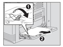
Check beneath the transport guide inside of the side cover. Check if any paper is misfed under the transport guide behind the transfer unit.
