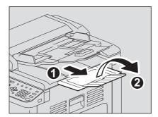
• To prevent misfeeding, do not leave originals or turn OFF/ON the equipment with originals on the Reversing Automatic Document Feeder.
