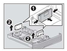
4 Attach the side guides according to the paper size.
