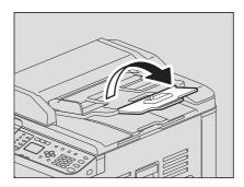
To prevent long originals (A3, B4, A4-R, LD, LG, COMP, or 8K) from sliding out, extend the paper exit stopper and raise the sub-stopper. When you have finished using the stopper, lift it slightly and slide it back in.
