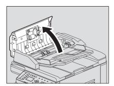
Open the transport guide and remove the original.
