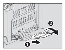
• When using thick paper for bypass copying, some thick paper may not be fed properly. In this case, turn over the paper and place it again as shown in the figure.
