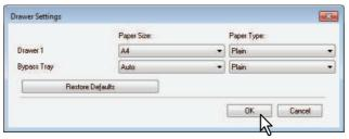
Drawer 1 — Select the size of paper that is loaded in the Drawer. The paper type for the drawer is fixed
