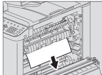
Return the transport guide and transfer unit to their original positions, and then close the side cover.
