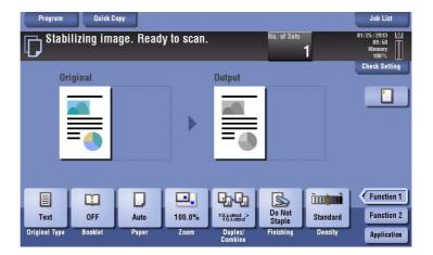
Image stabilization is performed while a large number of copies are being output or the temperature or humidity inside the machine has changed.
