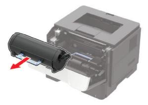
**3** Remove the used imaging unit.
