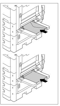
3 Slide the Lateral Guide to fit the size of paper being loaded.
