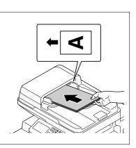
3 Slide the adjustable Lateral Guide against the edges of the original.
