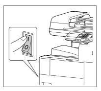
2 To turn the power off, press () on the **Power Switch**.
