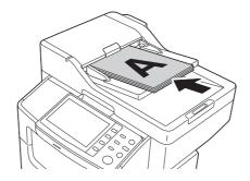
→ Load the original so that its top side is placed at the back. When loading in a different orientation, be sure to specify the loading direction of originals.
