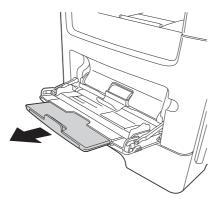
**3** Fully pull out the extension guide of the **Manual Feed Tray**.
