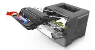
**Warning—Potential Damage:** Do not touch the shiny blue photoconductor drum under the imaging unit. Doing so may affect the quality of future print jobs.
