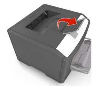
To open the paper stop, pull it so that it flips forward.
