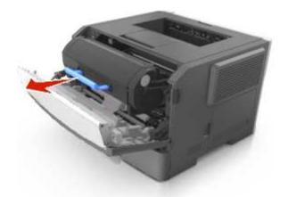
3. Lift the blue handle, and then pull the imaging unit out of the printer.
