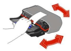
5. Remove all packing materials from the imaging unit.
