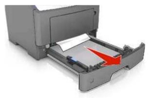
2. Firmly grasp the jammed paper on each side, and then gently pull it out. Note: Make sure all paper fragments are removed.
