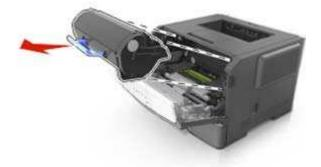
3. Lift the green handle, and then pull out the imaging unit from the printer.
