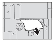
4 If it is difficult to find or remove the jammed paper, open the drawer of the Paper Feed Unit.
