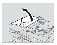
**5** Raise the original feeder tray, and remove the original under the tray.
