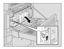
**10** Remove the transfer charger cleaner from the front pocket of the transfer unit.
