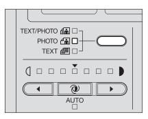
The automatic copy density mode, which automatically selects the most suitable density level for the copied image by detecting that of the original, is set by default at the installation of the equipment. You can also adjust the density level as desired manually (=manual copy density mode) in the following procedure:
