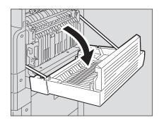
**9** Pull the transfer unit toward you carefully to lay it down while holding up the green lever.
