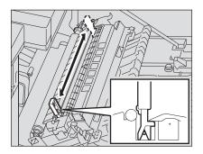
**5** Return the transfer charger cleaner into the cleaner pocket, and then close the transfer unit.
