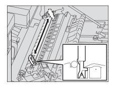
**12** Return the transfer charger cleaner into the cleaner pocket, and then close the transfer unit.
