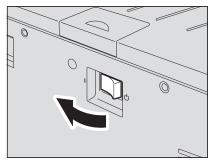
The equipment starts warming itself up. The warm-up time takes approx. 25 seconds. When the warm-up has finished, the equipment is ready for copying. "READY" appears on the LCD screen.
