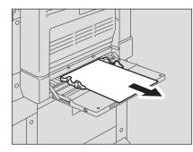
2 Check beneath the transport guide in the paper feeding area. Check if any paper is jammed under the transport guide behind the transfer unit. P.183 "Paper jam behind transfer unit"
