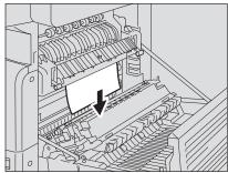
4 Return the transport guide to its original position, and then close the transfer unit and the side cover.
