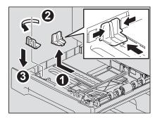
**5** Move the end guide to the trailing edge of the paper while pushing its lower part in the direction of the arrows.
