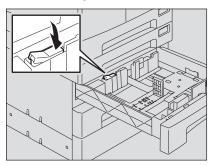
4 While pushing the green knob of the side guides, adjust the side guides at the position of the desired paper size.
