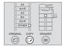
Press the selecting buttons (Center, Right) to select the size of the paper placed in the drawer. This can also be done with the ▲ or
