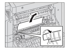
**5** If it is difficult to find or remove the jammed paper, open the drawer of the equipment.
