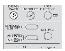
Check that the equipment is in the ready status, and press the [ENERGY SAVER] button.
