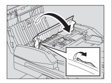
**5** Raise the guide plate under the transport guide, and remove the original under the guide plate.
