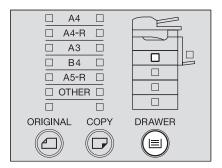
3 Press the [COPY] button several times until the lamp of the paper size you placed in the drawer is lit.
