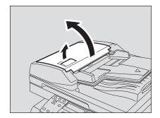
5 Raise the original feeder tray, and remove the original under the tray.
