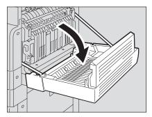
2 Pull the transfer unit toward you carefully to lay it down while holding up the green lever.
