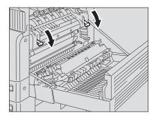
2 Open the transport guide while holding the knob.
