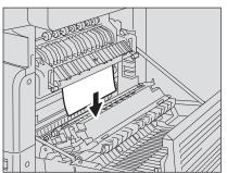
4 Return the transport guide to its original position, and then close the transfer unit and the side cover.
