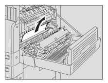
4 Open the transport guide of the paper feeding area and check if any paper is jammed under this guide. Clear the paper if there is any.
