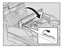
5 Raise the guide plate under the transport guide, and remove the original under the guide plate.
