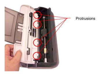
4. Insert two protrusions in the middle of the ADF Paper Tray into the holes on the top of the scanner.
